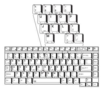
Figure 5-2 The numeric keypad overlay
